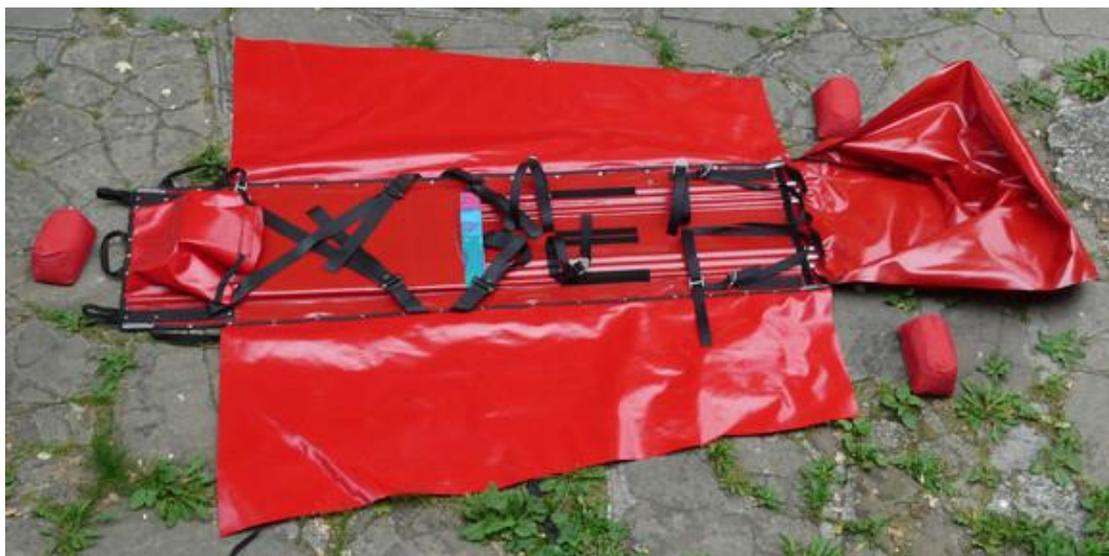
4. After the flaps are closed, the stretcher is tightened with 4 sets of external straps so that it forms a tube-like shape.
